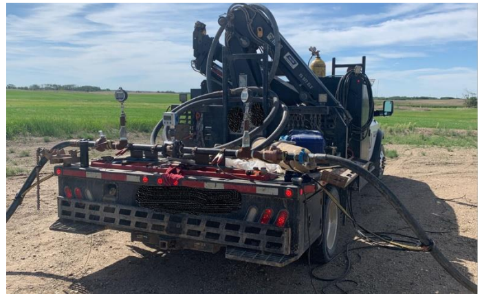
(c) Fluid withdrawal test setup showing the metering run
