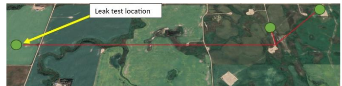
Figure 15 Pipeline Network considered for Case-3 showing pipeline carrying emulsions from two satellite sites to a separator.
