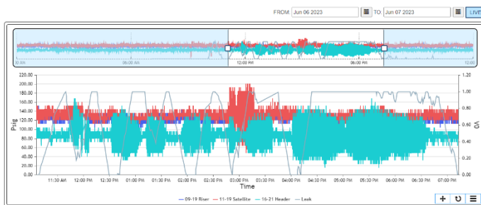
Figure 22 Pressure trends during the false positive leak alarms
